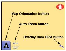
Press the Auto Zoom button to toggle the feature on and off. The Overlay Data Hide button will clear overlay data boxes from the map screen. Select it again to bring them back. Use the Map Orientation button to select between three different map views.
